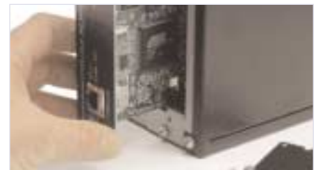
APC accessory cards can be inserted into the built-in SmartSlot to allow monitoring of power conditions. The Smart-UPS RT 5000, 7500, and 10,000 units ship bundled with the Web/SNMP Management Card
