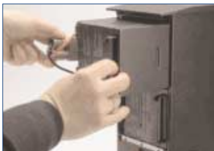
User-friendly, hot-swappable battery replacement
